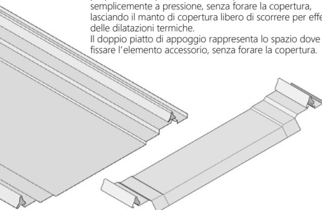
For the fastening of lightweight roofing accessories, such as finishing sheets and photovoltaic beams, Nav System offers an aluminium clip, which can be simply press-fitted, without drilling holes in the roofing, thus leaving the roofing membrane free to slide due to thermal expansion. The double support plate is the space where the accessory element can be fastened, without drilling holes in the roofing.
