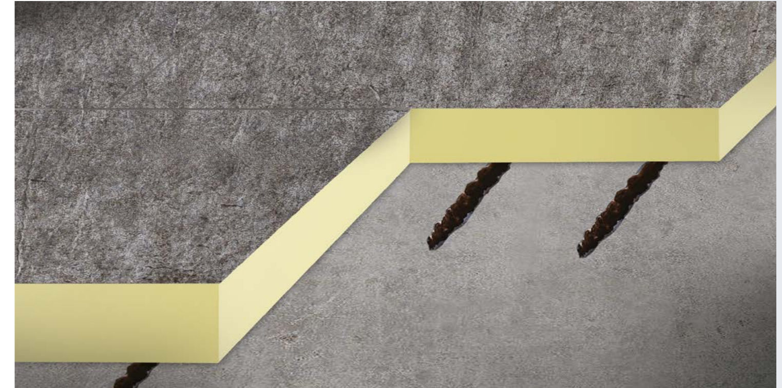
Adesione con collanti o schiuma poliuretanic / Bonding with adhesives or polyurethane foam
